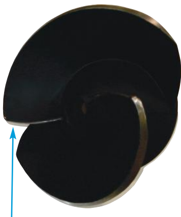
Modified vane profiles.
