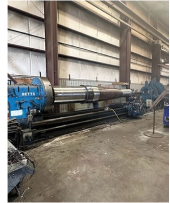
Horizontal lathe machining a crusher main shaft
