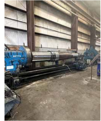
Horizontal lathe machining a crusher main shaft
