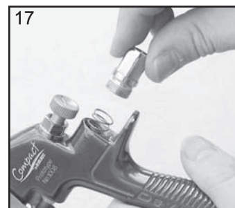
17. Replace Valve Spring and screw in Housing (10).
