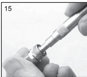
15. Fit Seal to Housing (10).
