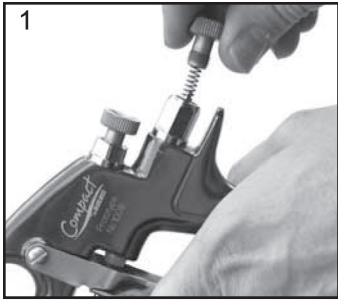
1. Remove Adjusting Knob (7), Spring (8), and Needle (9).
