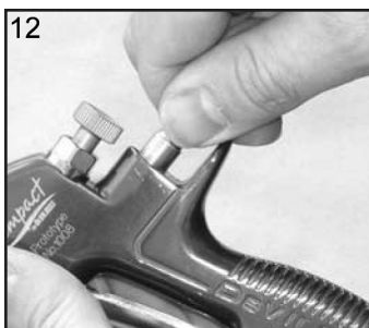
12. Fit Valve Seat to Gunbody.
