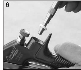
6. Remove Valve Seat.
