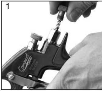
1. Remove Adjusting Knob (7), Spring (8), and Needle (9).
