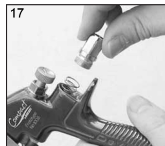
17. Replace Valve Spring and screw in Housing (10).
