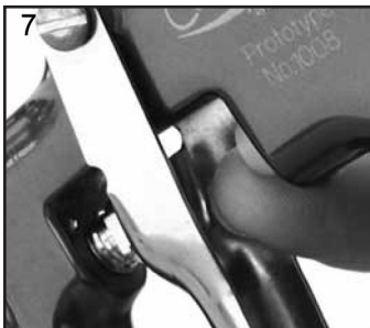
7. Push out the Front Air Valve Seal with a finger.
