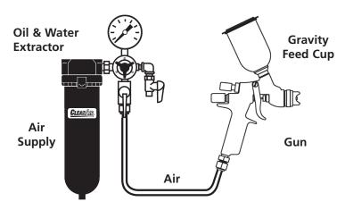
Air pressure for atomization is regulated at the extractor. The flow of the fluid is adjusted by the fluid valve control knob on gun, viscosity of paint and air pressure.
